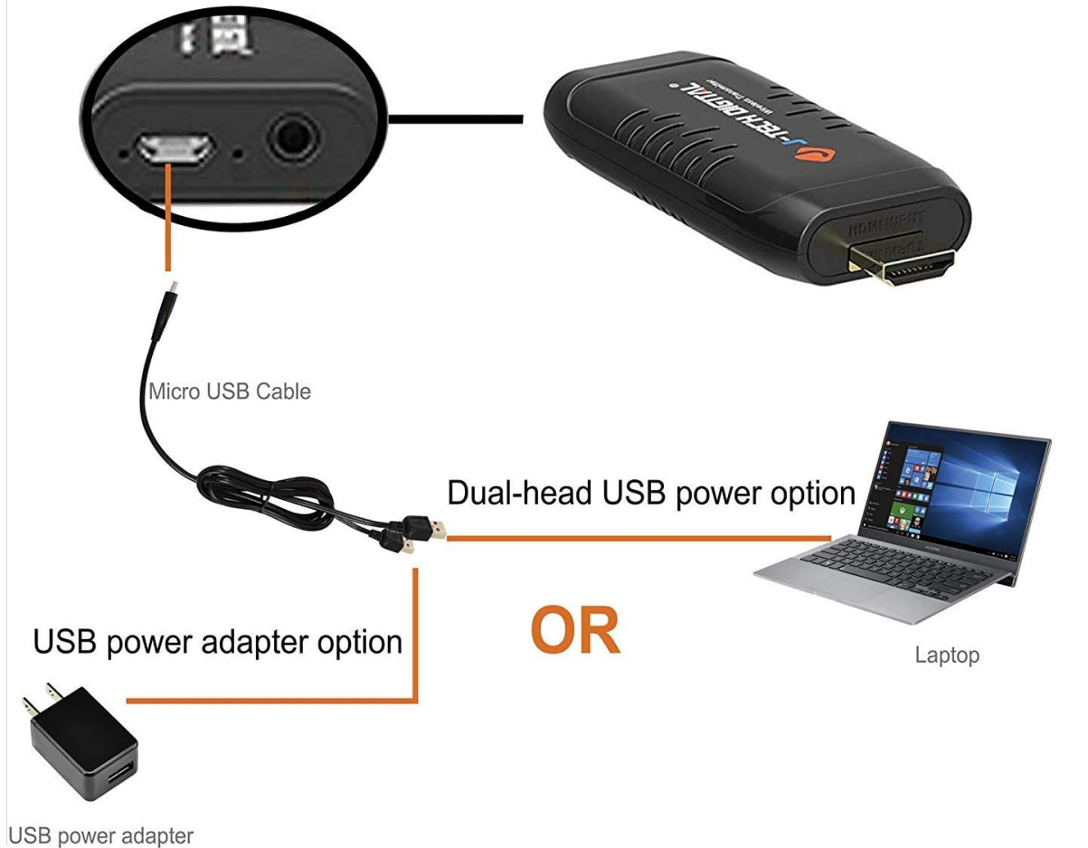
Figure 4.1: Various power supply options for the J-Tech Digital Wireless HDMI Extender, including USB power adapter or laptop USB port.
