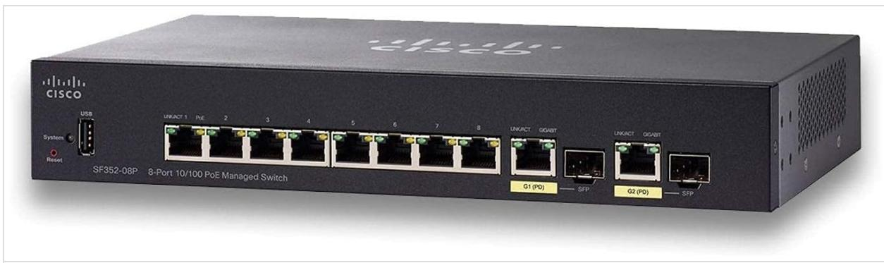
This image displays the front panel of the Cisco SF352-08P Managed Switch. From left to right, it features a USB port, System and Reset buttons, eight 10/100 PoE Ethernet ports with corresponding Link/Act and PoE status LEDs, and two Gigabit Ethernet (GbE) combo SFP ports (G1 and G2) with their own Link/Act LEDs. The model number 'SF352-08P 8-Port 10/100 PoE Managed Switch' is printed below the ports.
