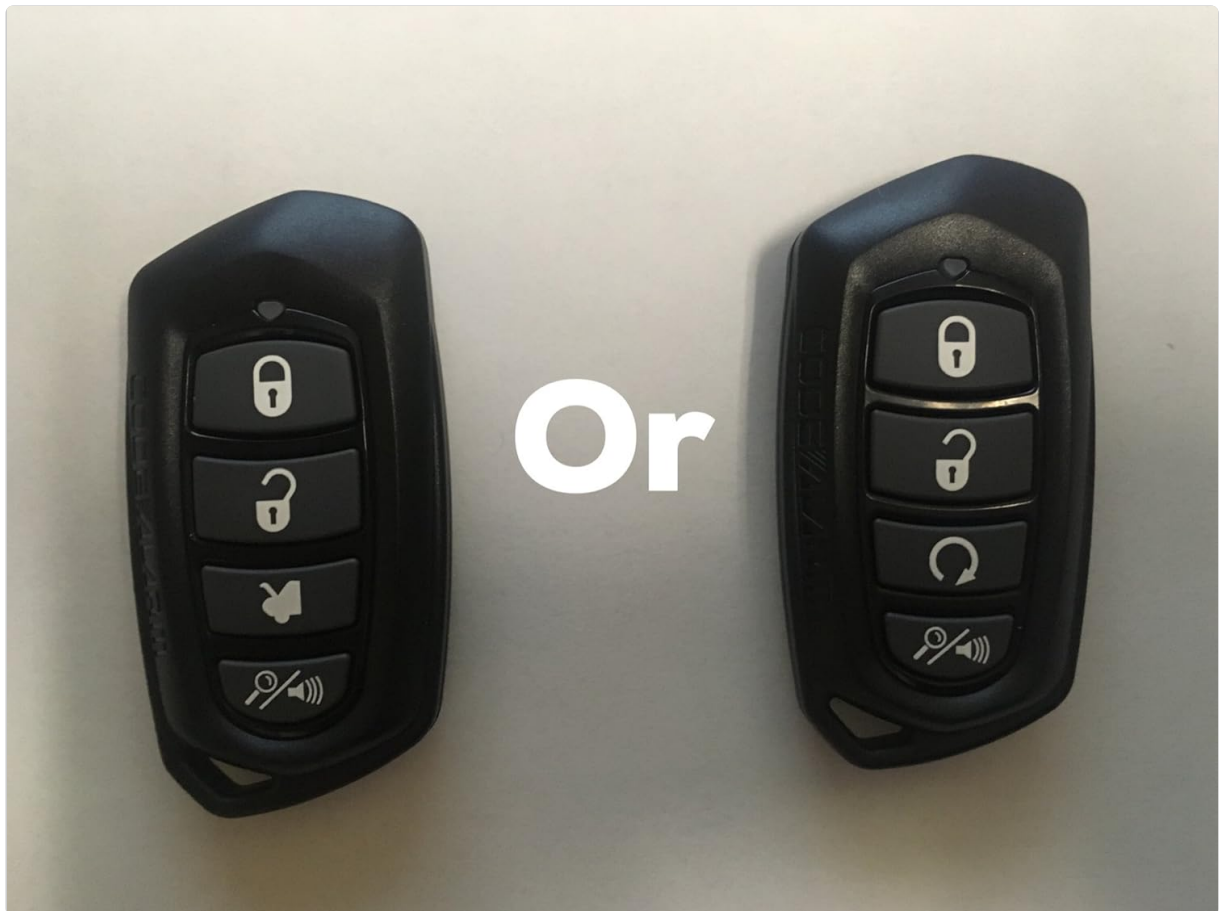
Image: Two variations of the Code Alarm CAT4P replacement remote. Both are black, oval-shaped, and feature four gray buttons. The left remote includes a trunk release icon, while the right remote features a circular arrow icon for remote start. This illustrates the slight variations in button configuration for the same model.
