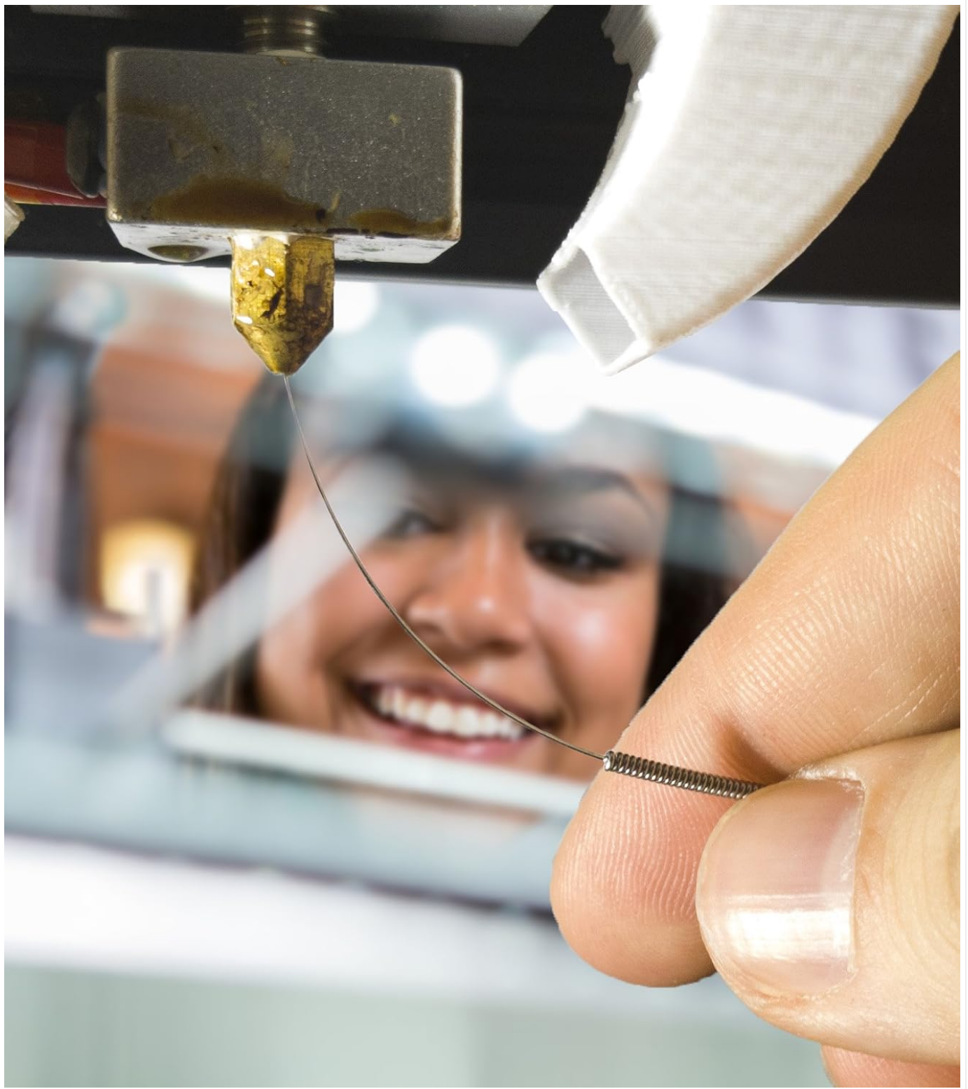
Figure 3: Demonstrates the careful insertion of a 0.40mm cleaning needle into a 3D printer nozzle to clear blockages.
