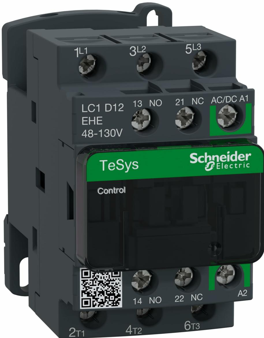
Figure 1: Front view of the LC1D12EHE Contactor, showing main power terminals (1L1, 3L2, 5L3, 2T1, 4T2, 6T3), auxiliary contacts (13 NO, 14 NO, 21 NC, 22 NC), and coil terminals (A1, A2).
