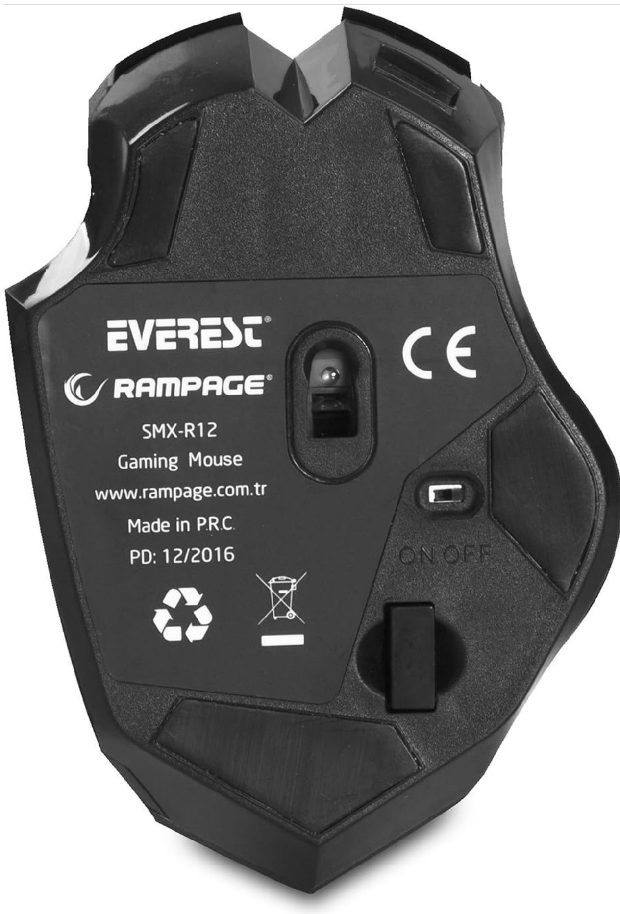
Figure 2.3: Bottom view of the Rampage SMX-R12 Hawker Gaming Mouse, showing the optical sensor, On/Off switch, and USB receiver storage compartment.
