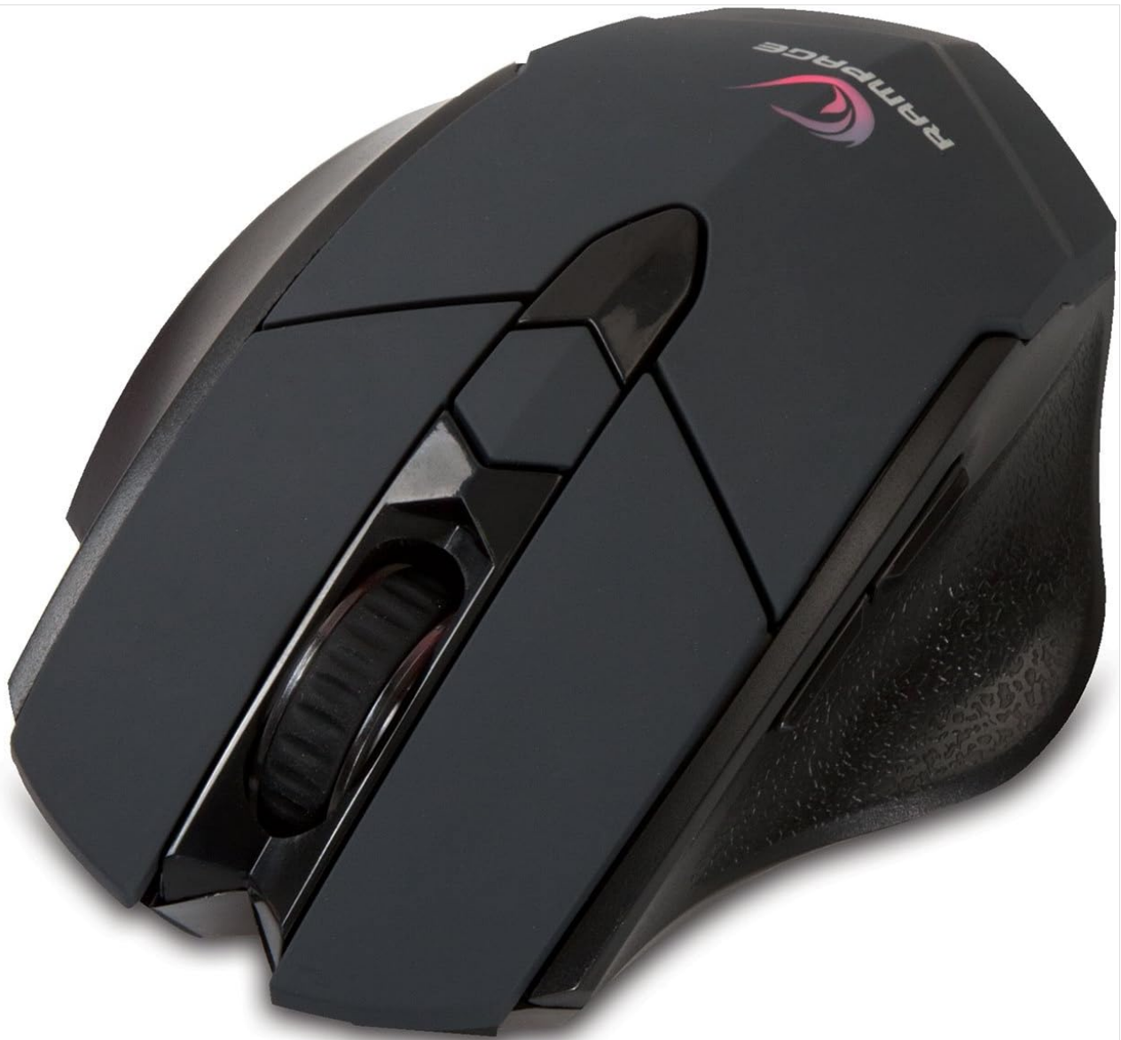
Figure 2.1: Top view of the Rampage SMX-R12 Hawker Gaming Mouse, showing the left/right click buttons, scroll wheel, and DPI adjustment buttons.
