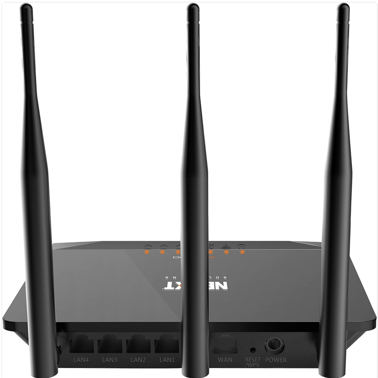
Image 4.1: Rear view of the Amp300 highlighting the WAN, LAN, Reset/WPS, and Power ports.
