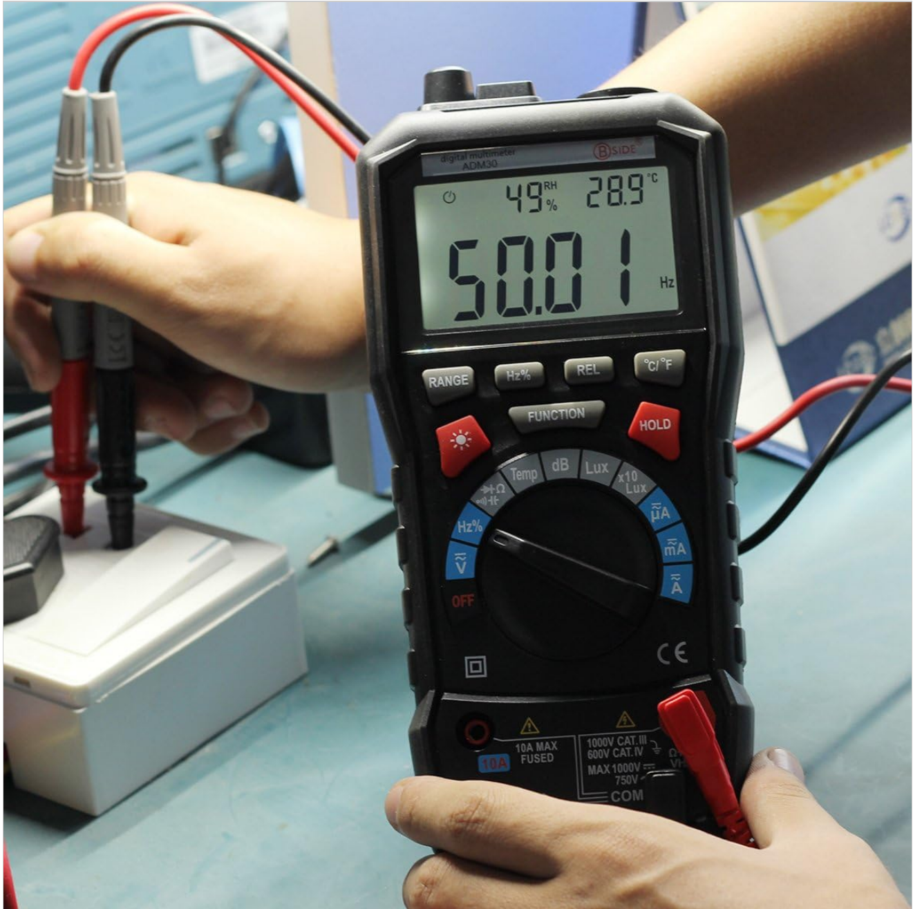
Figure 4.3: The multimeter displaying a frequency measurement.
