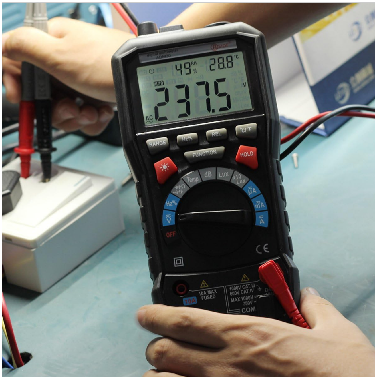
Figure 4.1: The multimeter displaying an AC voltage measurement from a power outlet.
