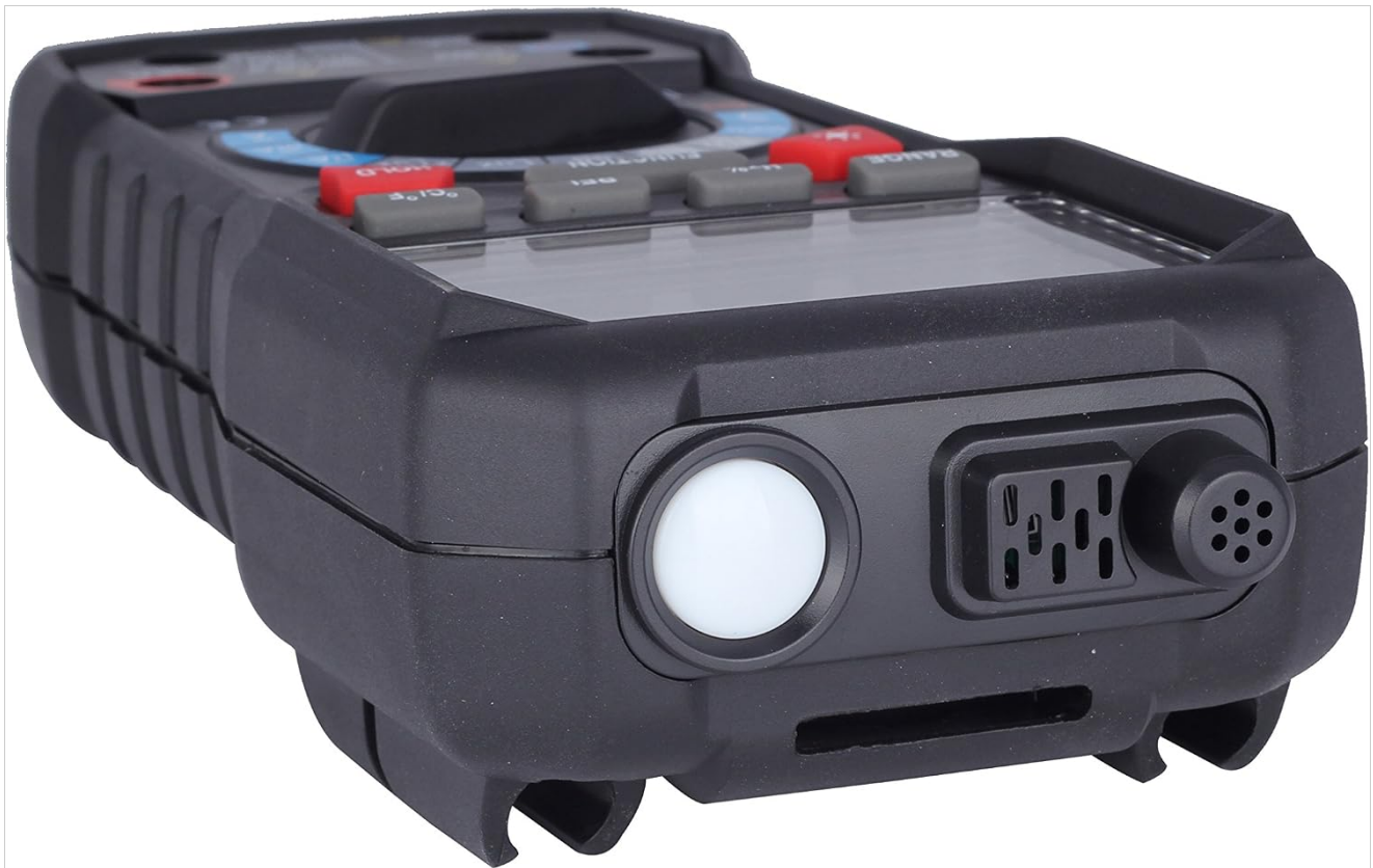
Figure 4.4: Side view of the multimeter, highlighting the integrated light and sound sensors.
