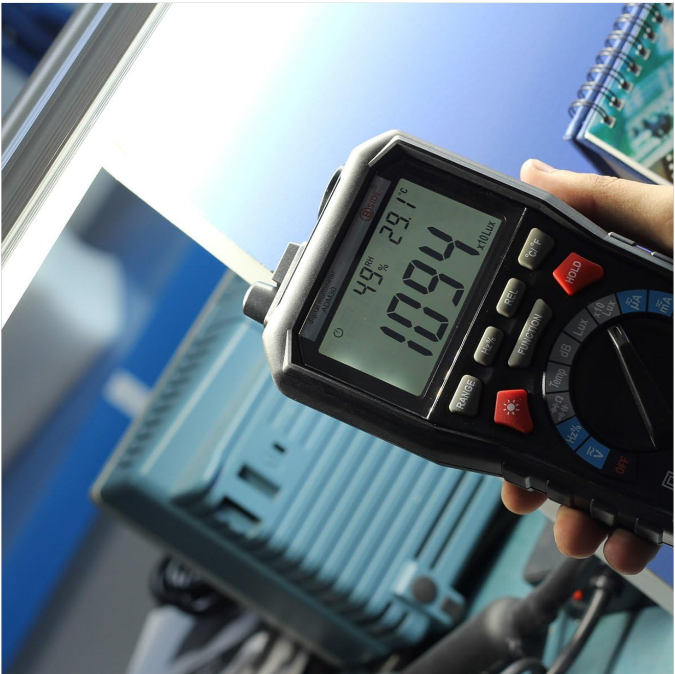
Figure 4.5: The multimeter displaying a luminance measurement in Lux.
