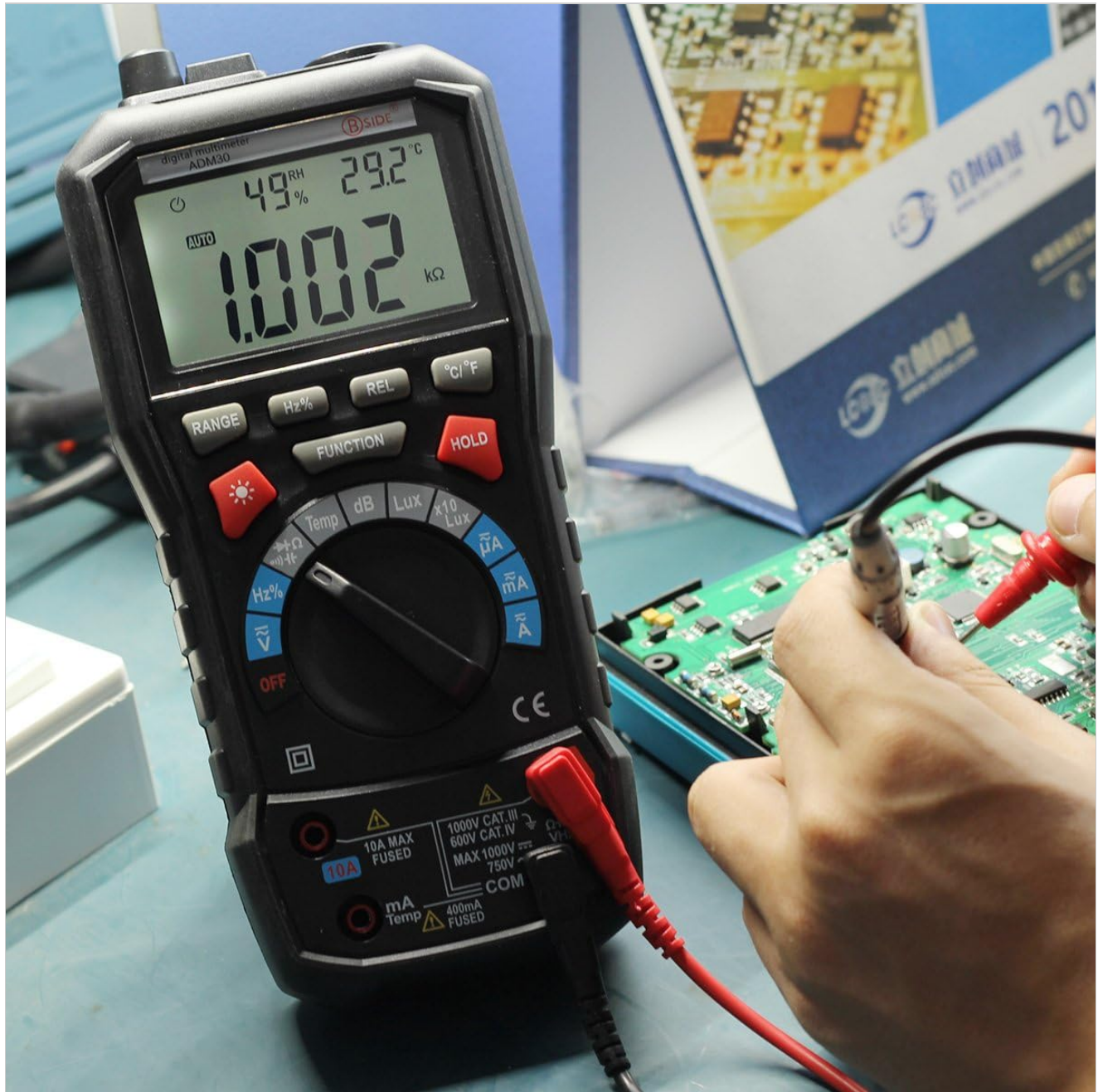
Figure 4.2: The multimeter displaying a resistance measurement on a circuit board.
