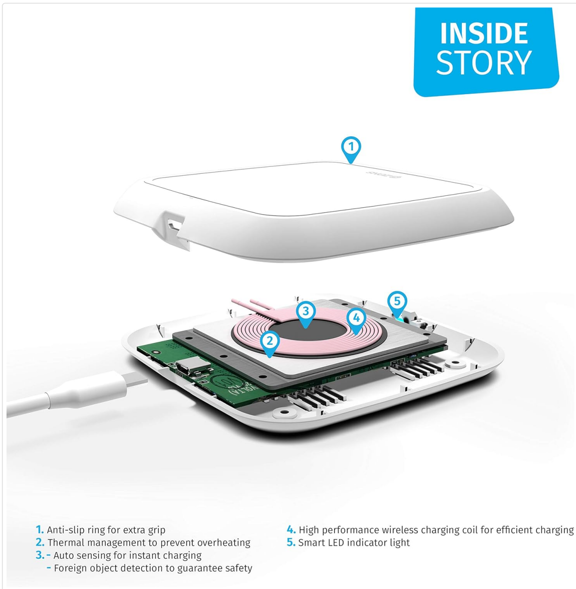
Image 4: Internal components and their functions within the charging pad.
