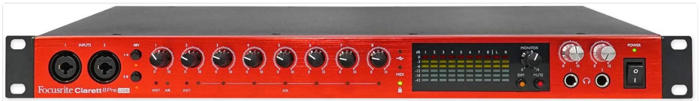
Figure 2: Front Panel Overview. This image shows the front panel of the Clarett 8Pre USB, highlighting the input jacks, gain knobs, and metering display.
