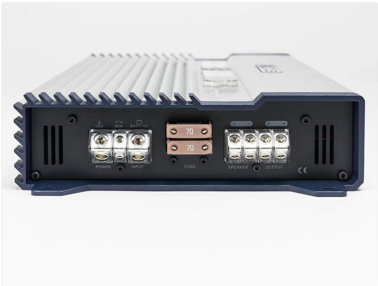
Image: Rear view of the Hifonics BXX1600.1D amplifier. This image highlights the power input terminals (+12V, REM, GND) on the right, and the mono speaker output terminals on the left. Two 70A fuses are visible between the power and speaker terminals, indicating the amplifier's power handling capabilities.
