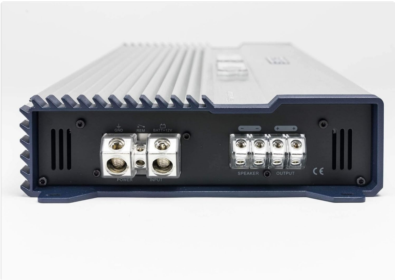
Image: Close-up view of the power input (GND, REM, BATT+12V) and speaker output terminals on the Hifonics BXX4000.1D amplifier. This image illustrates where to connect the main power, ground, remote, and speaker wires.
