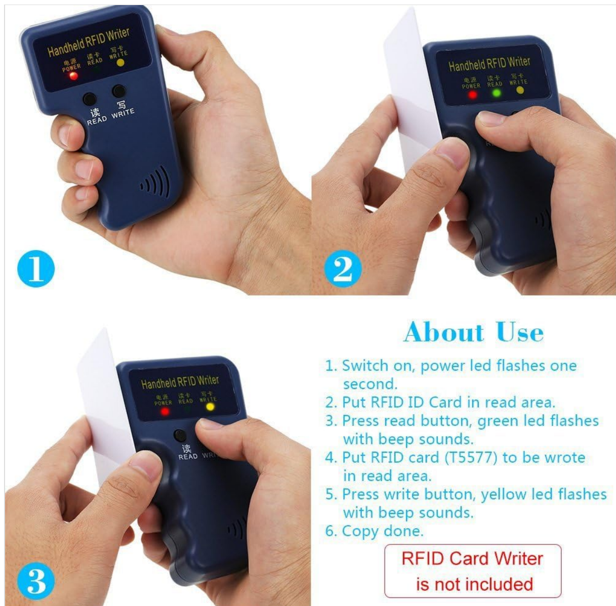
Image 3.1: A visual guide demonstrating the process of writing to an RFID card using a handheld RFID writer. The steps include powering on, placing the card, pressing read/write buttons, and confirming completion.
