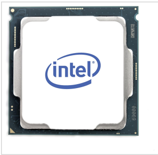
Image: Top view of the Intel Core i5-8600 processor, showing the IHS.
