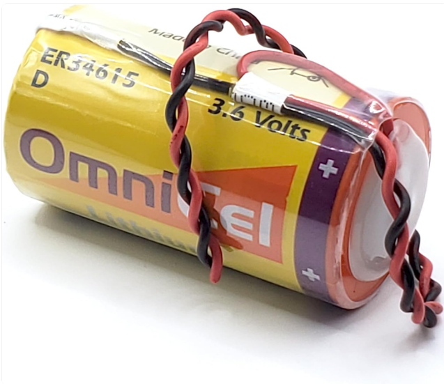
Figure 3.2: Detailed view of the battery's label, indicating "3.6 Volts" and model "ER34615 D", along with the twisted wire leads.
