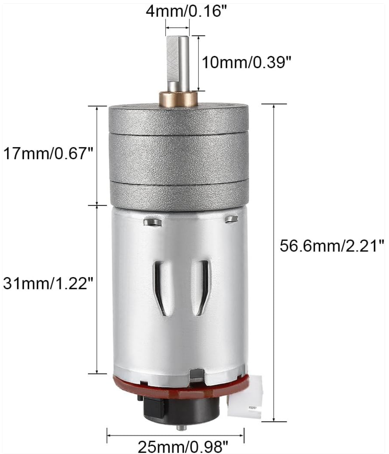
Figure 2: Detailed dimensions of the gear motor and shaft.
