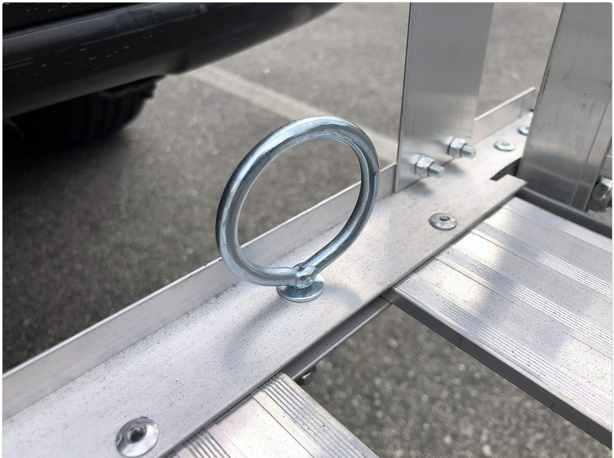
Figure 4.2: Anti-wobble bracket installed to reduce carrier movement.
