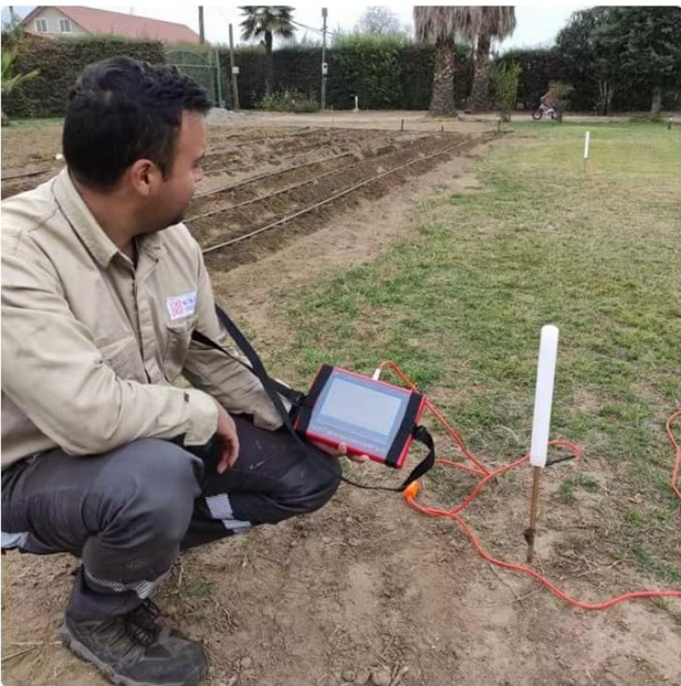
Image 3.1: Proper connection of the electrode cable to the main unit.
