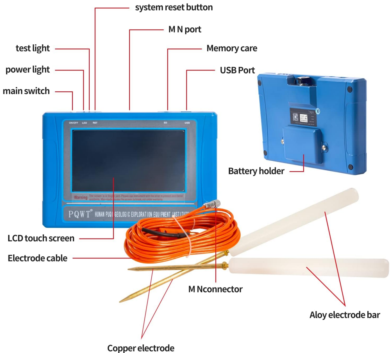
Image 2.1: Labeled components of the PQWT-TC500 Ground Water Detector.
