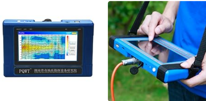
Image 4.1: Examples of data visualization on the PQWT-TC500's LCD screen.
