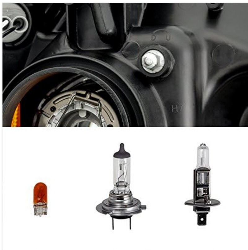
Image 6.1: Rear view of headlight showing bulb access and bulb types.
