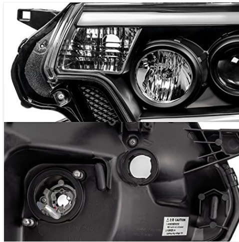
Image 4.1: Front and rear view of the headlight assembly.
