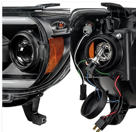
Image 4.2: Projector lens and rear wiring detail.
