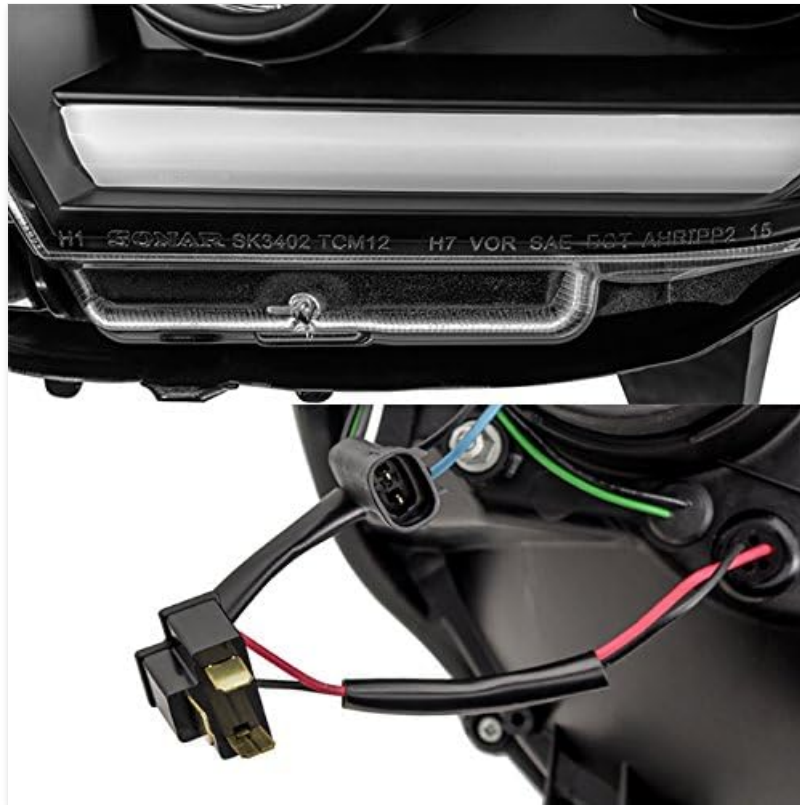
Image 4.3: LED DRL strip and wiring connections.
