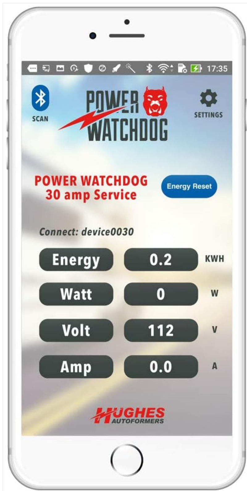
Figure 3: Close-up view of the Power Watchdog mobile application interface, showing real-time power data.
