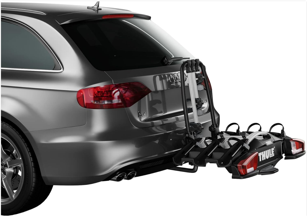
Image 4.3: The Thule VeloCompact bike rack tilted to allow access to the vehicle's trunk.
