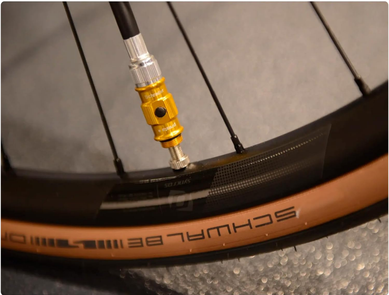
Figure 6: The ABS Flip Chuck securely connected to a bicycle tire valve, ready for inflation.
