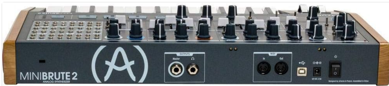
Image: Rear view of the MiniBrute 2, showing the power input, audio outputs, USB port, and MIDI In/Out connections.
