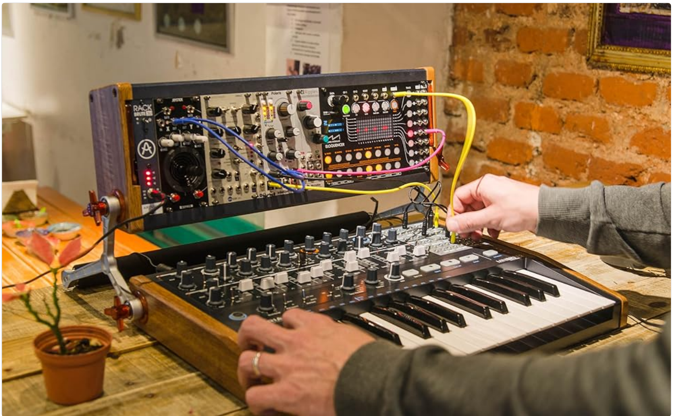
Image: Close-up of the MiniBrute 2's 48-point patchbay, showing various input and output jacks for modular connections.
