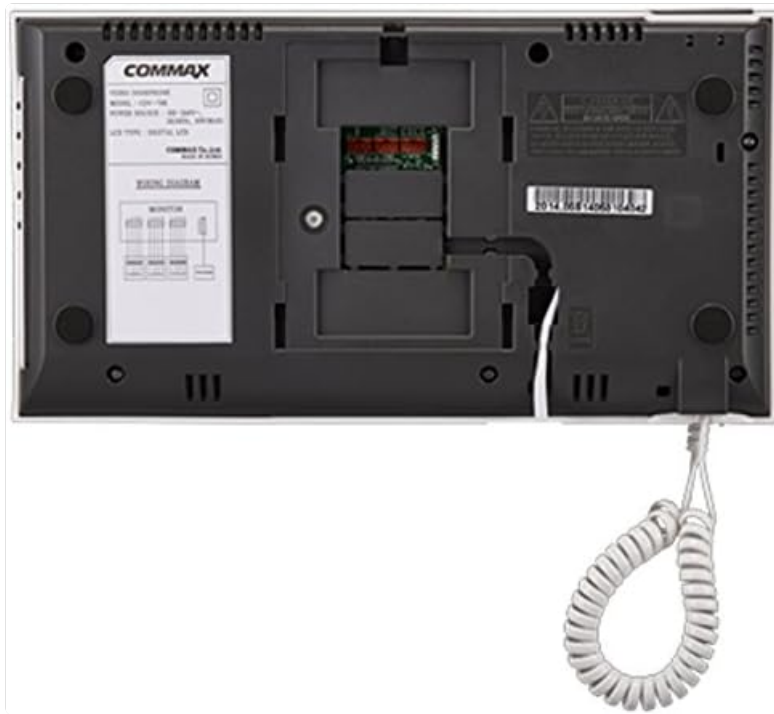
Figure 3: Rear view of the CDV-70K monitor, showing the wiring terminals and diagram.
