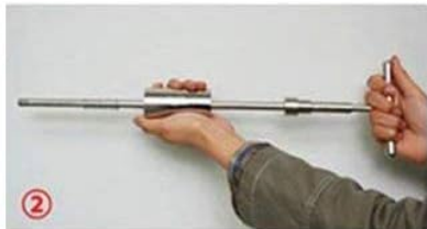
Image 3.1: Visual guide demonstrating the assembly steps for both the short and long configurations of the T-bar slide hammer.
