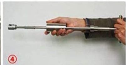
Image 3.1: Visual guide demonstrating the assembly steps for both the short and long configurations of the T-bar slide hammer.
