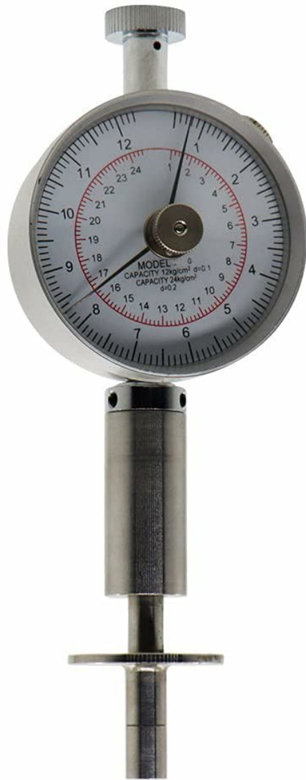
Figure 4: The tester's dial with inner and outer scales for different indenter sizes.
