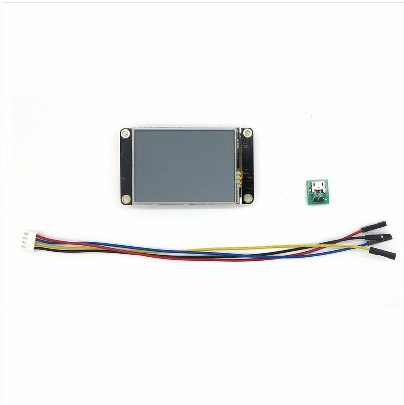
Figure 1: NEXTION NX4832K035 3.5-inch HMI touchscreen display module.
