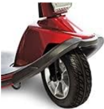
Image: Close-up of the front wheel and fender, showing the non-scuffing tire.
