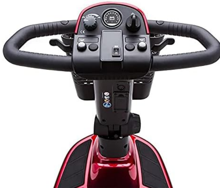
Image: Close-up view of the tiller control panel, showing the easy-grip adjustment knob, battery gauge, and other operational controls.
