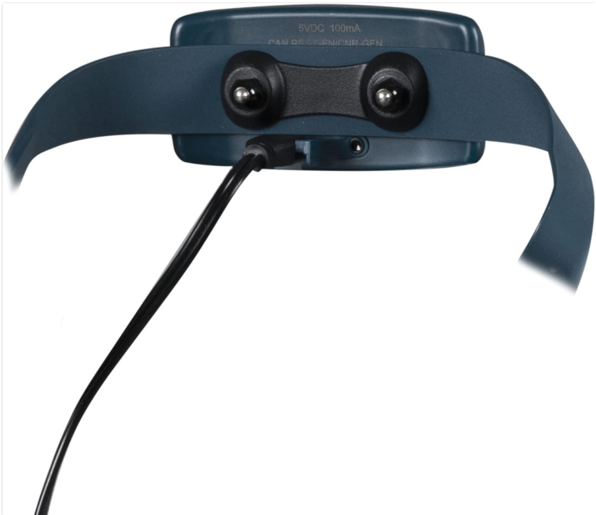
Image: A close-up view showing the charging plug of the USB adaptor securely inserted into the charging port of a PetSafe remote trainer collar.
