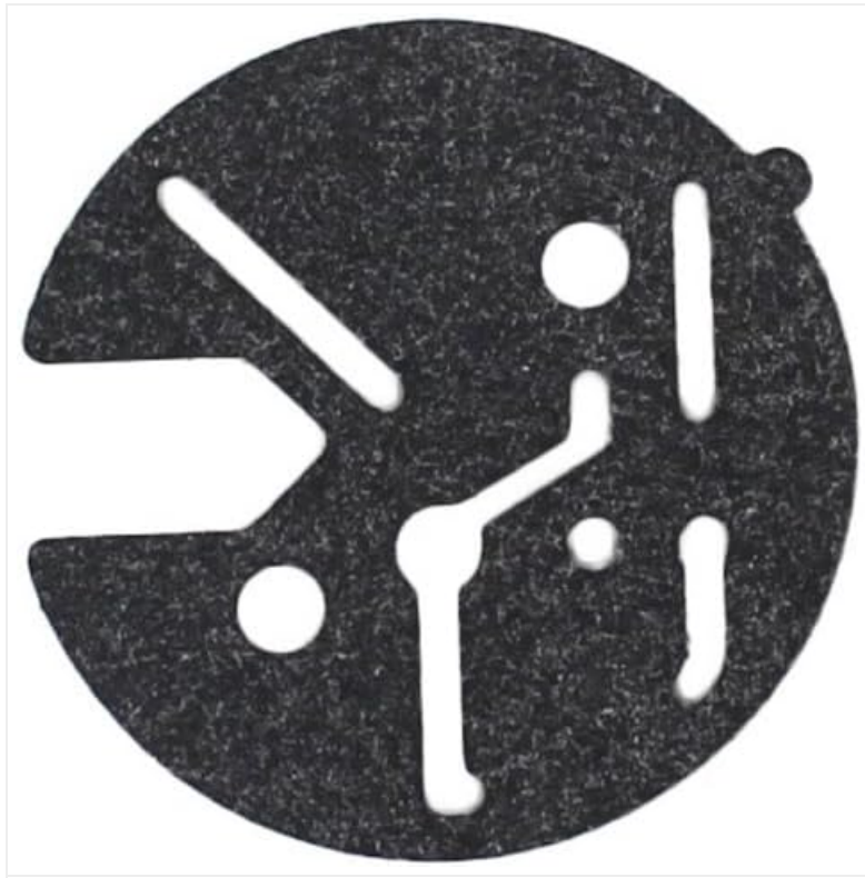
Image: Another circular diaphragm, often functioning as a fuel pump diaphragm.
