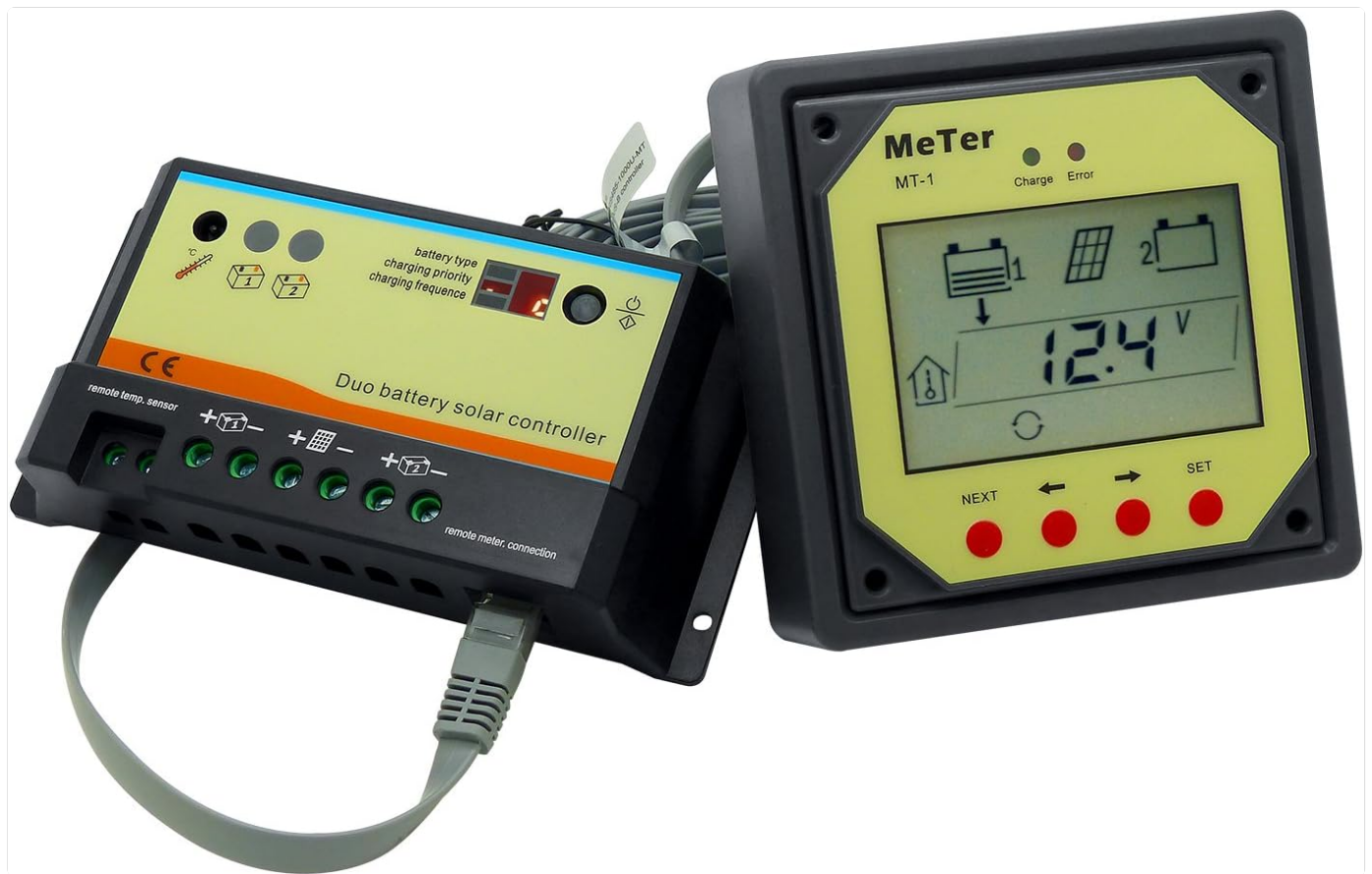
Figure 2: The EPIPDB-COM 20A controller connected to the MT-1 remote meter via the communication cable.
