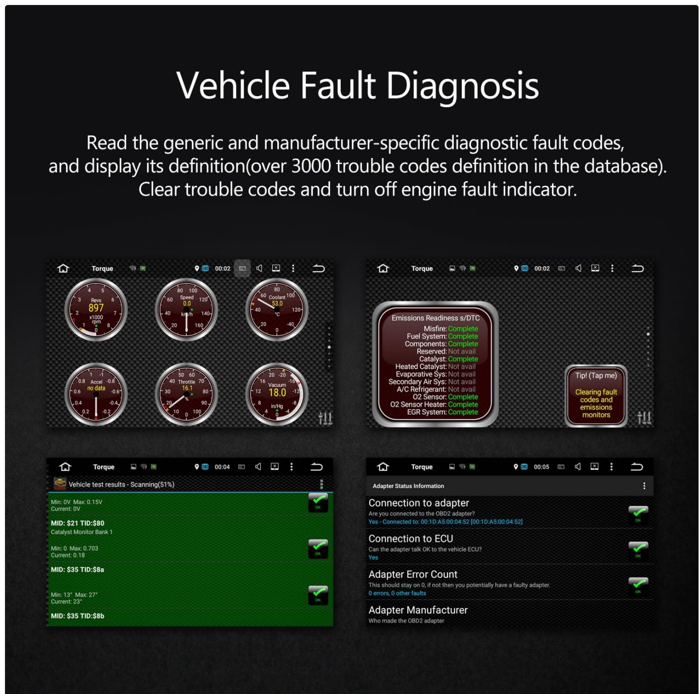
Image 5.1: The Torque app interface displaying vehicle fault diagnosis results and emissions readiness status.
