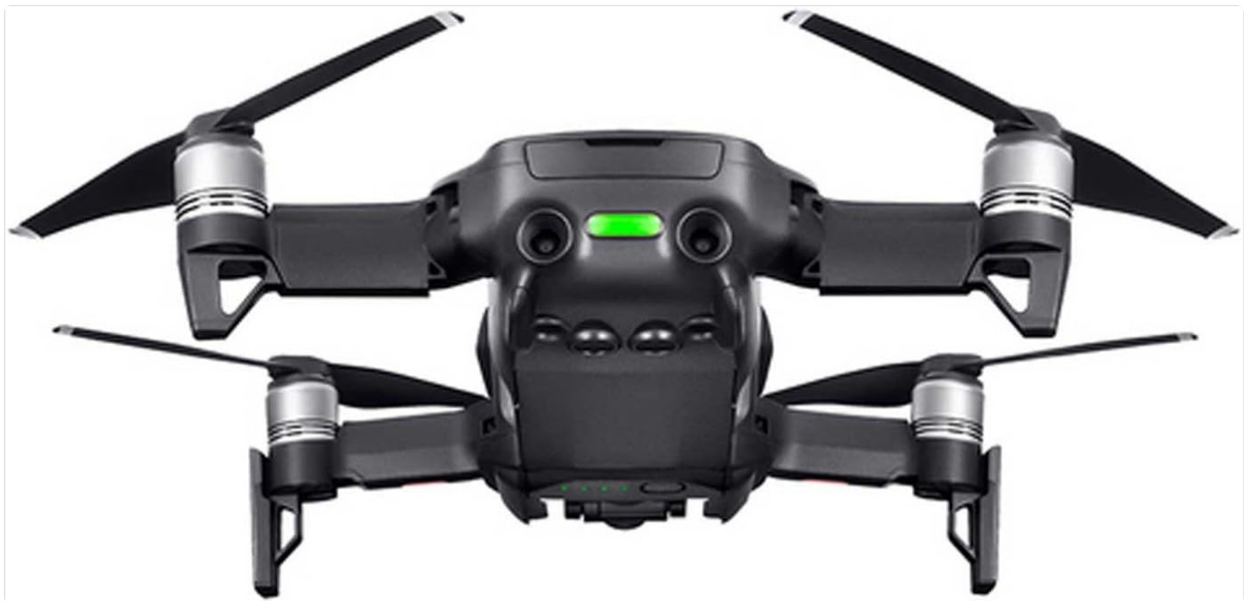
Figure 4.1: Rear view of the DJI Mavic Air drone, displaying the rear vision sensors.
