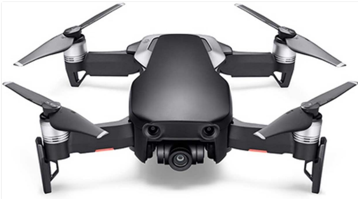
Figure 2.1: Front view of the DJI Mavic Air drone, showcasing its camera and forward sensors.
