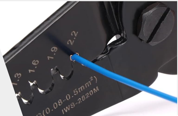
Image 3.1: Visual guide for the crimping process. Step 1 shows paralleling pin barrels, Step 2 shows inserting the terminal into the jaw, and Step 3 illustrates crimping conductor and insulation tabs separately.
