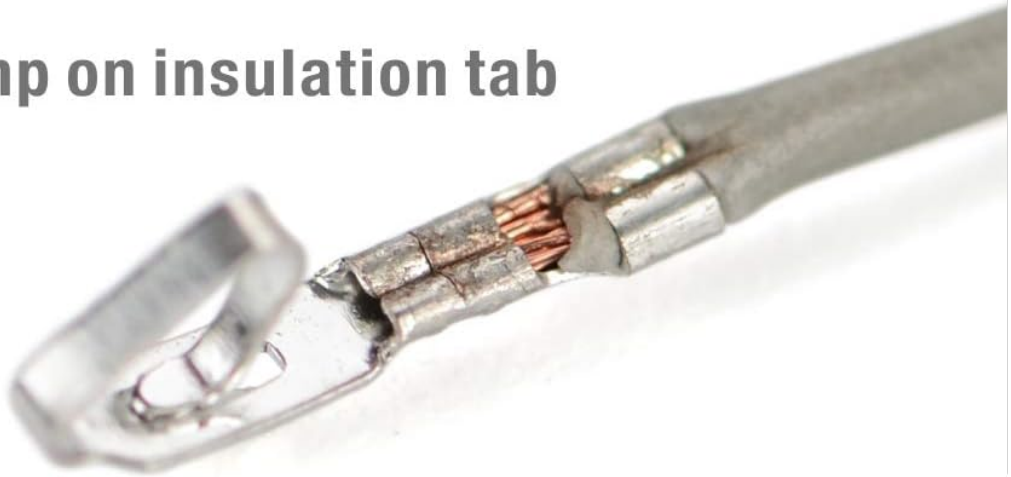
Image 3.3: Another example of a correctly crimped terminal on a grey wire, demonstrating the two-step crimping for conductor and insulation.
