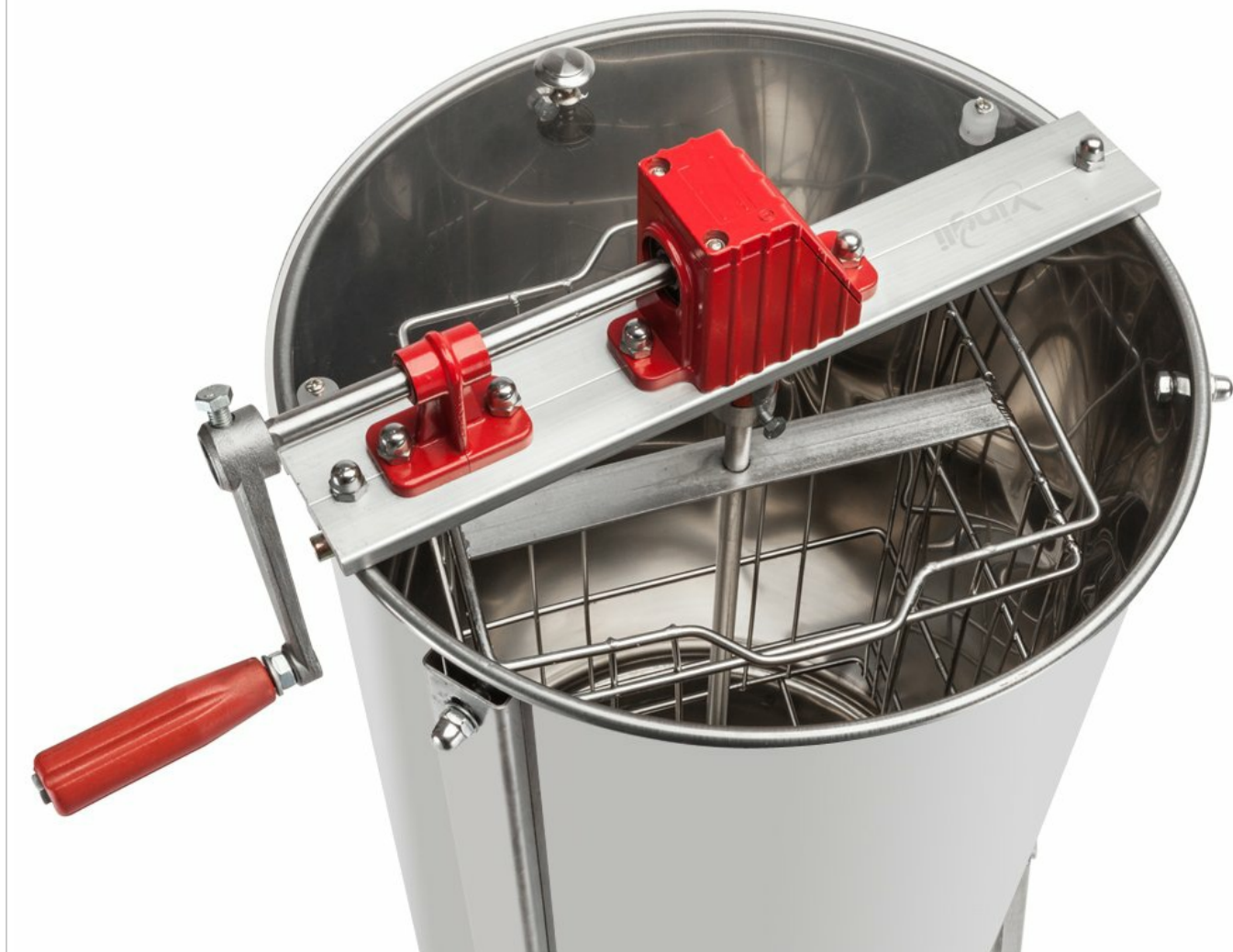
Figure 5.2: Top view of the extractor, showing the manual crank mechanism and the clear lid for observing the process.
