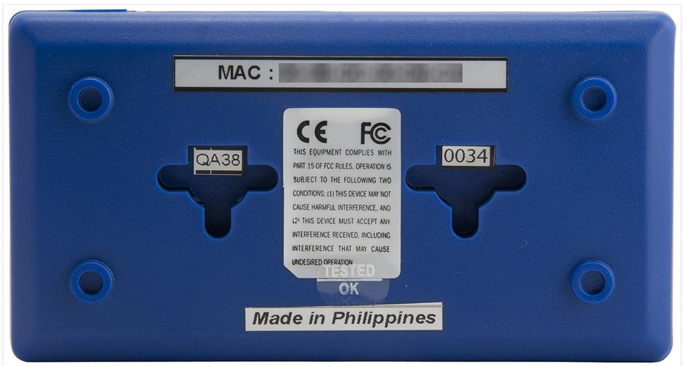
Figure 2.3: Bottom view of the SensorProbe2, displaying the MAC address label, CE and FCC regulatory compliance markings, and "Made in Philippines" text.
