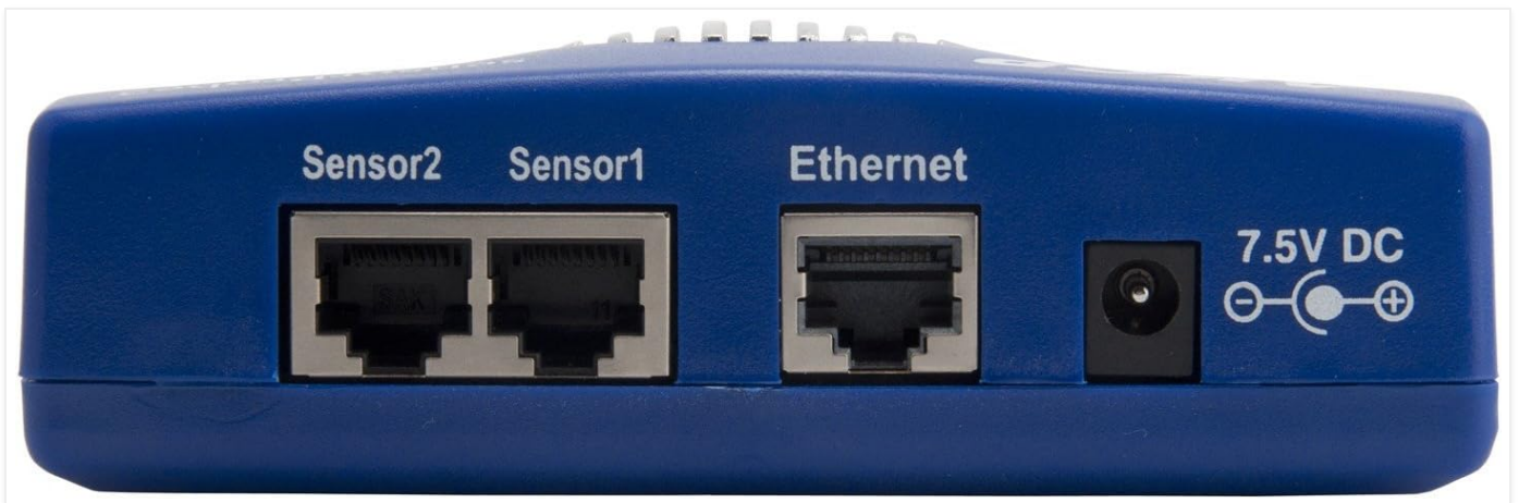
Figure 2.2: Rear view of the SensorProbe2, detailing the two sensor ports (Sensor 1, Sensor 2), the Ethernet port, and the 7.5V DC power input.
