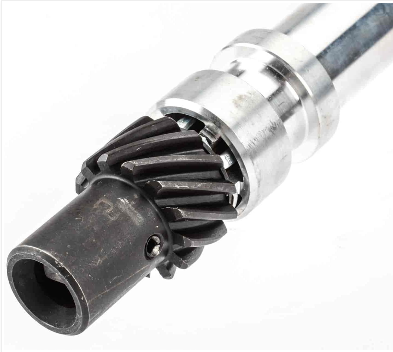
Figure 3: Close-up view of the standard-type steel distributor gear.
