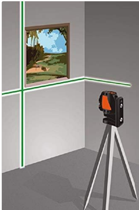
Figure 5.2: The laser level assisting in window installation, providing accurate horizontal and vertical references for proper alignment.
