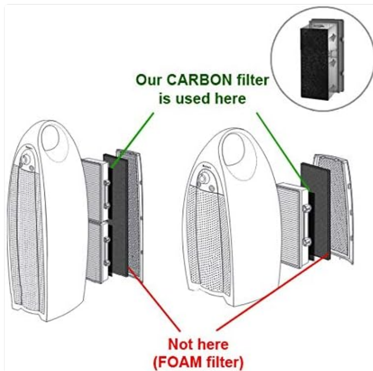
Image: Diagram illustrating the correct placement of the carbon filter within an air purifier, distinguishing it from the foam pre-filter.
