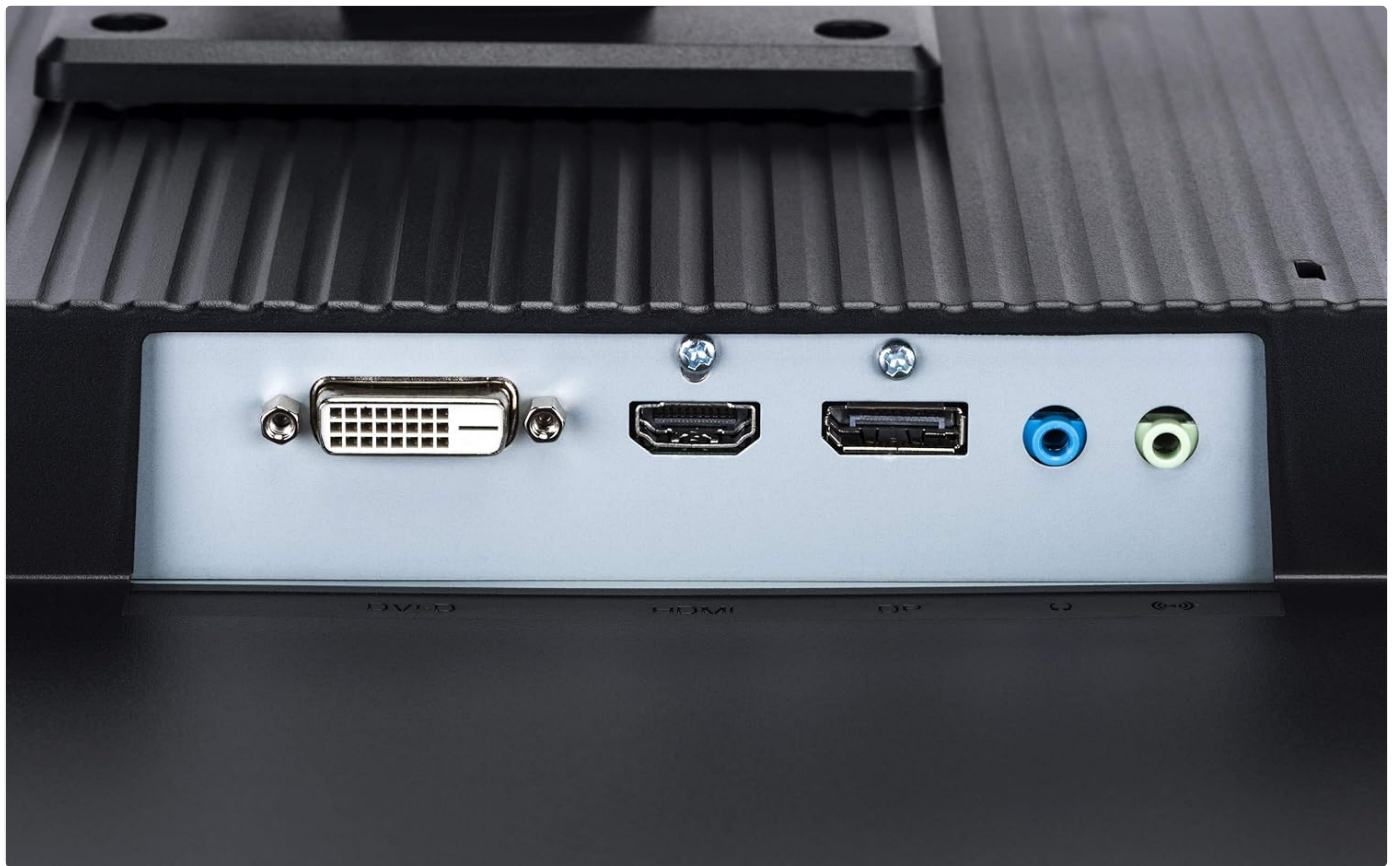
Figure 4: Detailed view of the monitor's input ports, including DVI, HDMI, DisplayPort, and audio connections.
