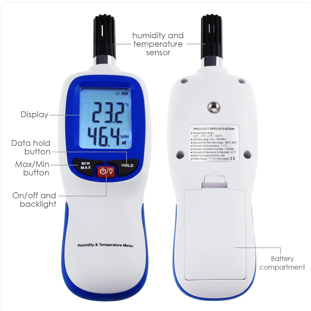
Image 2.1: Front and back view of the meter with labeled components. Key parts include the humidity and temperature sensor at the top, the LCD display, the Data Hold button, the Min/Max button, the On/Off and Backlight button, and the battery compartment on the rear.
