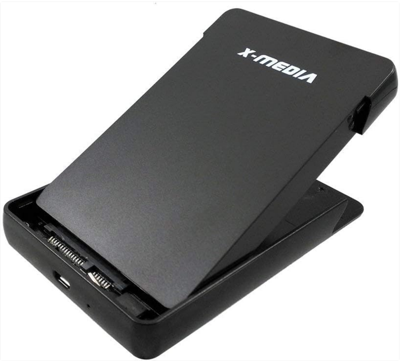
Image: The enclosure with the drive fully inserted and the cover being closed.
