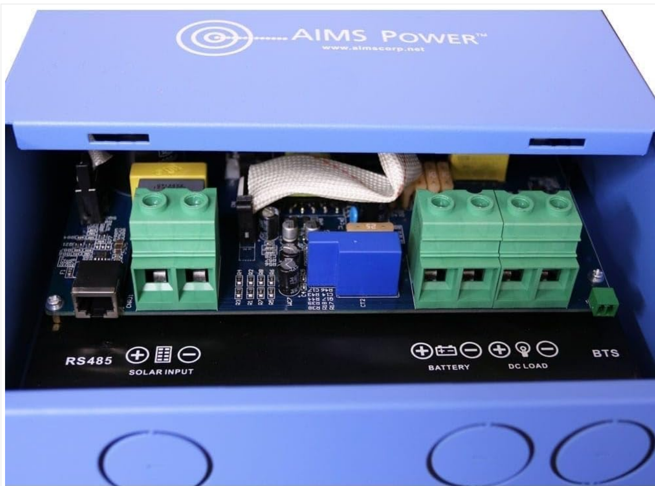
Figure 3: Internal view of the connection terminals.
