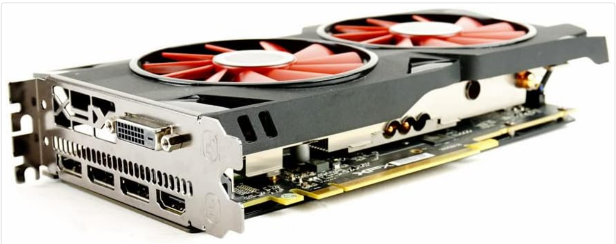
Figure 2: Angled view of the graphics card showing the dual fans and heatsink.
