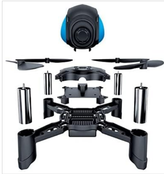
Image 4.1: Exploded view showing the main frame, motors, propellers, drone body, and canopy, illustrating how the Eclipse drone components fit together for assembly.
