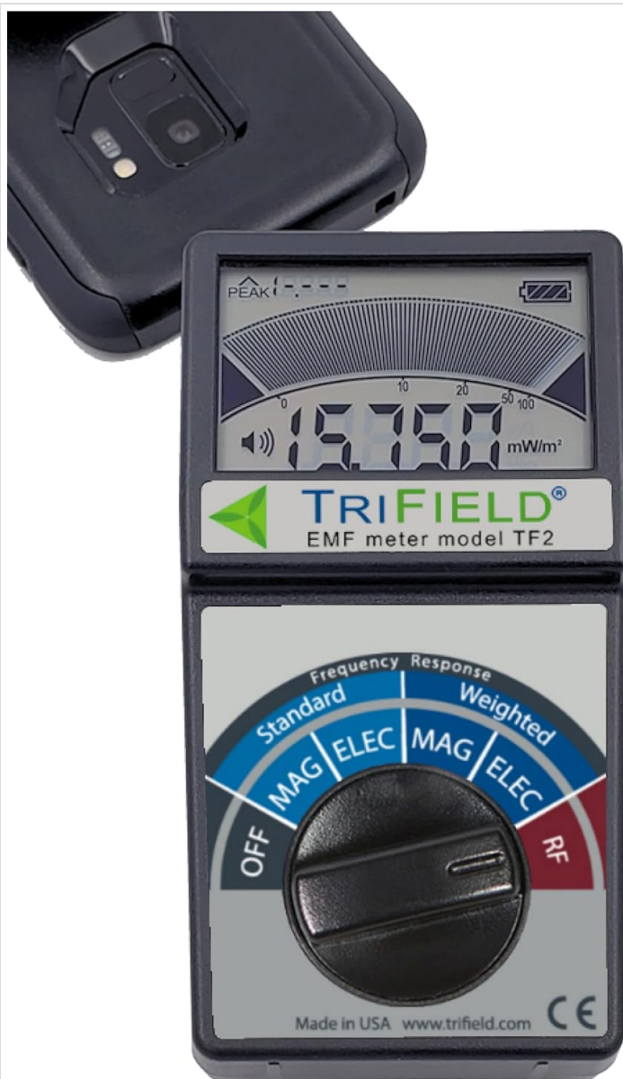
Figure 4.2: The TriField EMF Meter TF2 actively measuring radio frequency (RF) emissions from a nearby cell phone, displaying the current power density.
