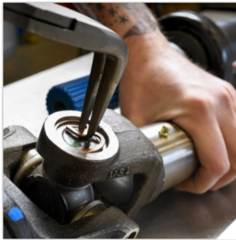
Figure 5: The serviceable design of Dorman U-joints allows for easier maintenance and replacement.
