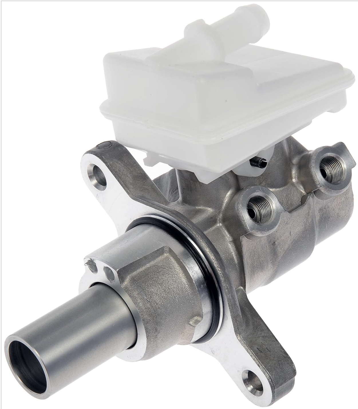
Image 5.1: Another view of the Dorman M630924 Brake Master Cylinder, showing the mounting points.
