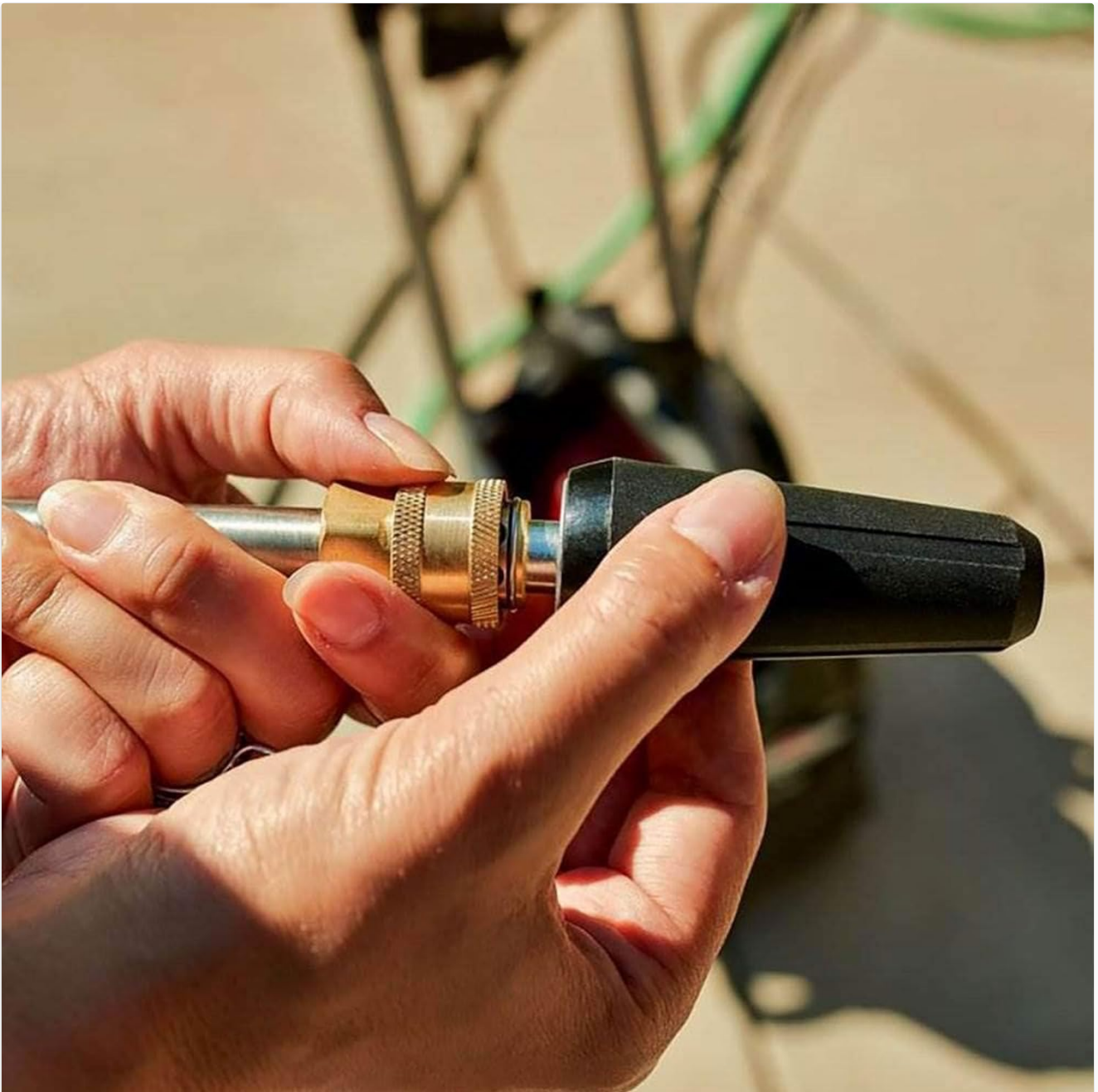
Image 4.1: Illustrates the process of connecting a spray nozzle to the wand.
