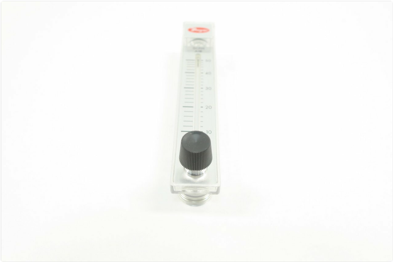
Figure 5: The adjustment knob located at the bottom of the flow meter, used for fine-tuning the flow rate if the meter is equipped with an integral valve.
